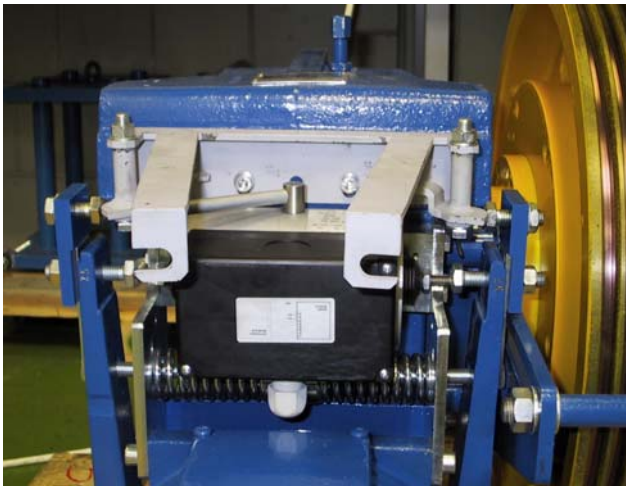
Fig. 15 : Remote linkage for remotely opening the Brake Levers.
