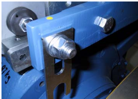
Fig 11: Loosened Brake Spring Pressure Screw
